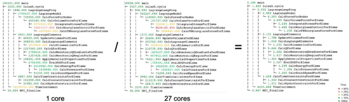
Figure 4: HATCHET’s ‘division’ operator enables calculation of speedup in each function in the application via a single line in a Python script, quickly pinpointing bottlenecks. HATCHET trees shown demonstrate Lulesh execution on (a) 1 core, (b) 27 cores, and (c) the speedup of 1/27 cores.
